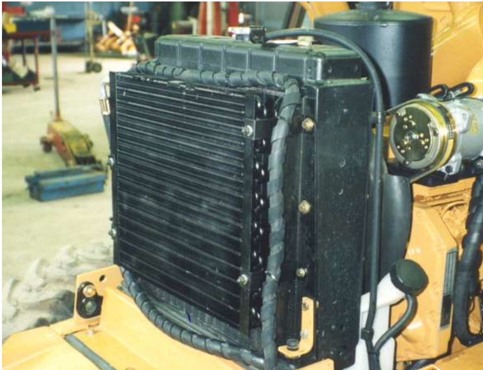
Condenser in place with left side brackets and hose routing shown.
