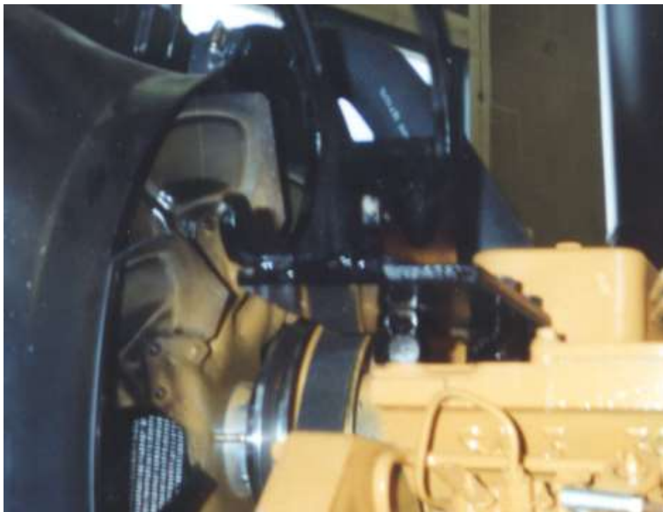
Compressor mount with stand-offs on engine.
