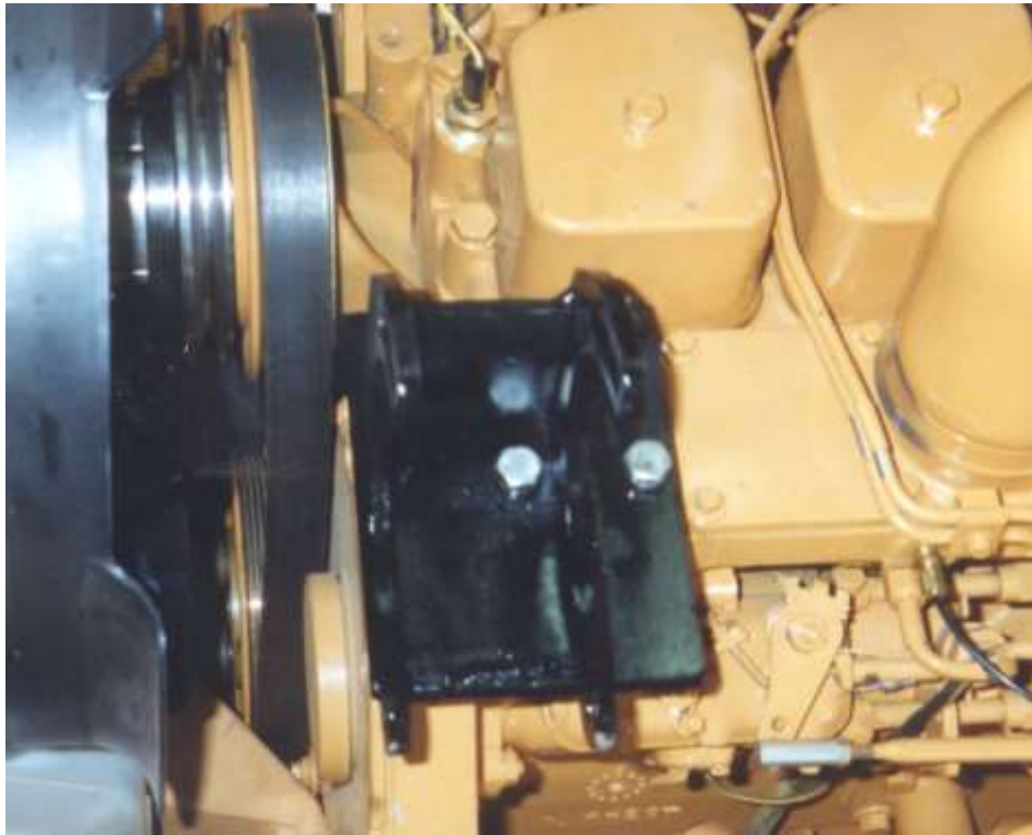
Compressor mount location on engine.
