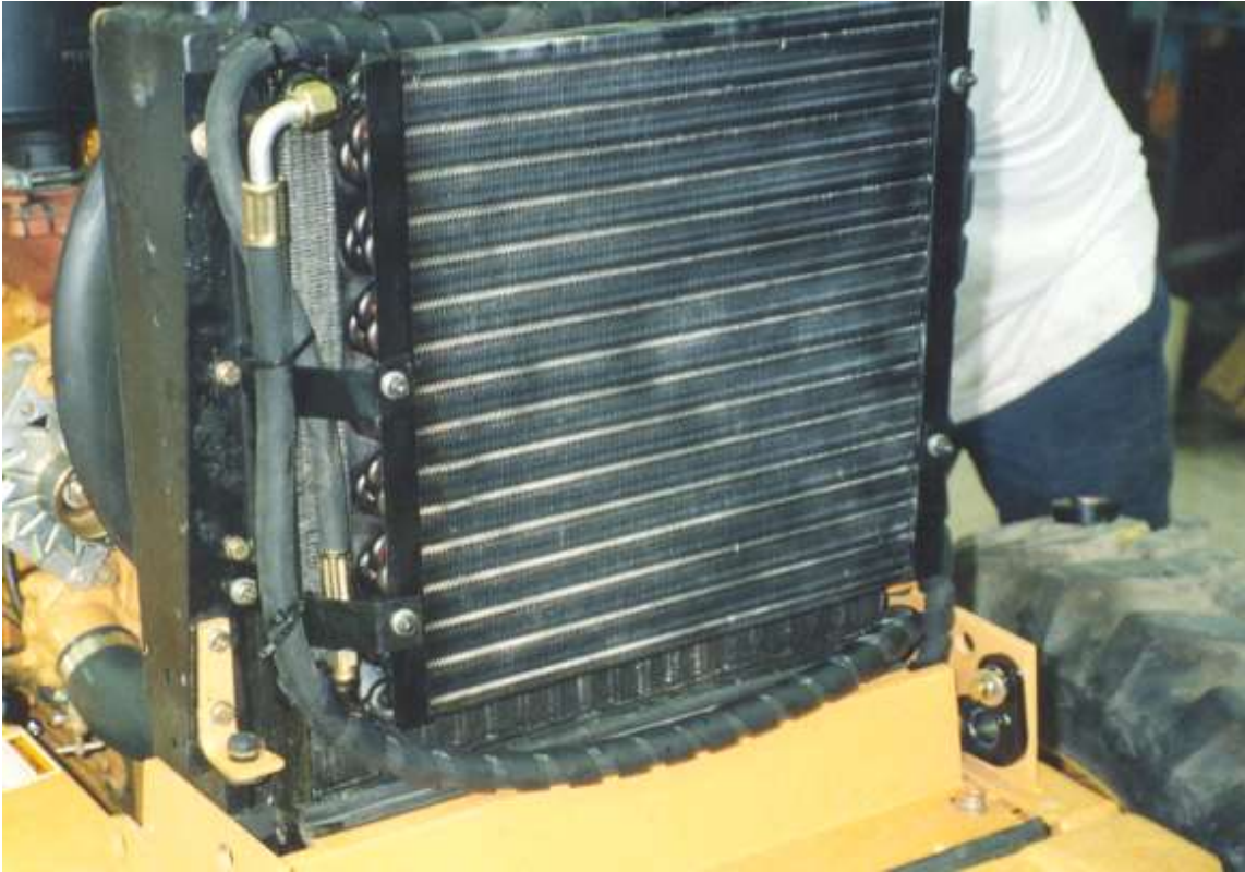
Condenser mounted with hoses in place showing right side brackets.
