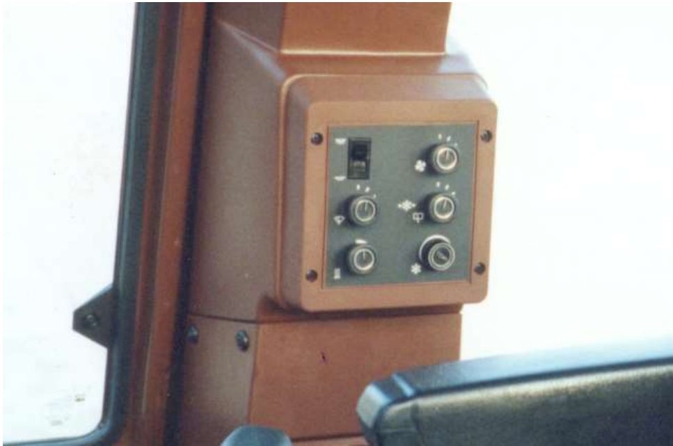
Thermostat in position on lower right of panel.
