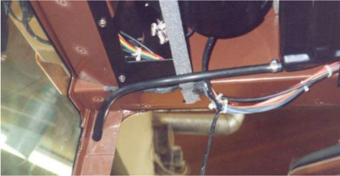
Drain tube to front column.
