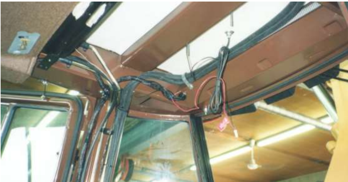
Hose routing in cab from evaporator.
